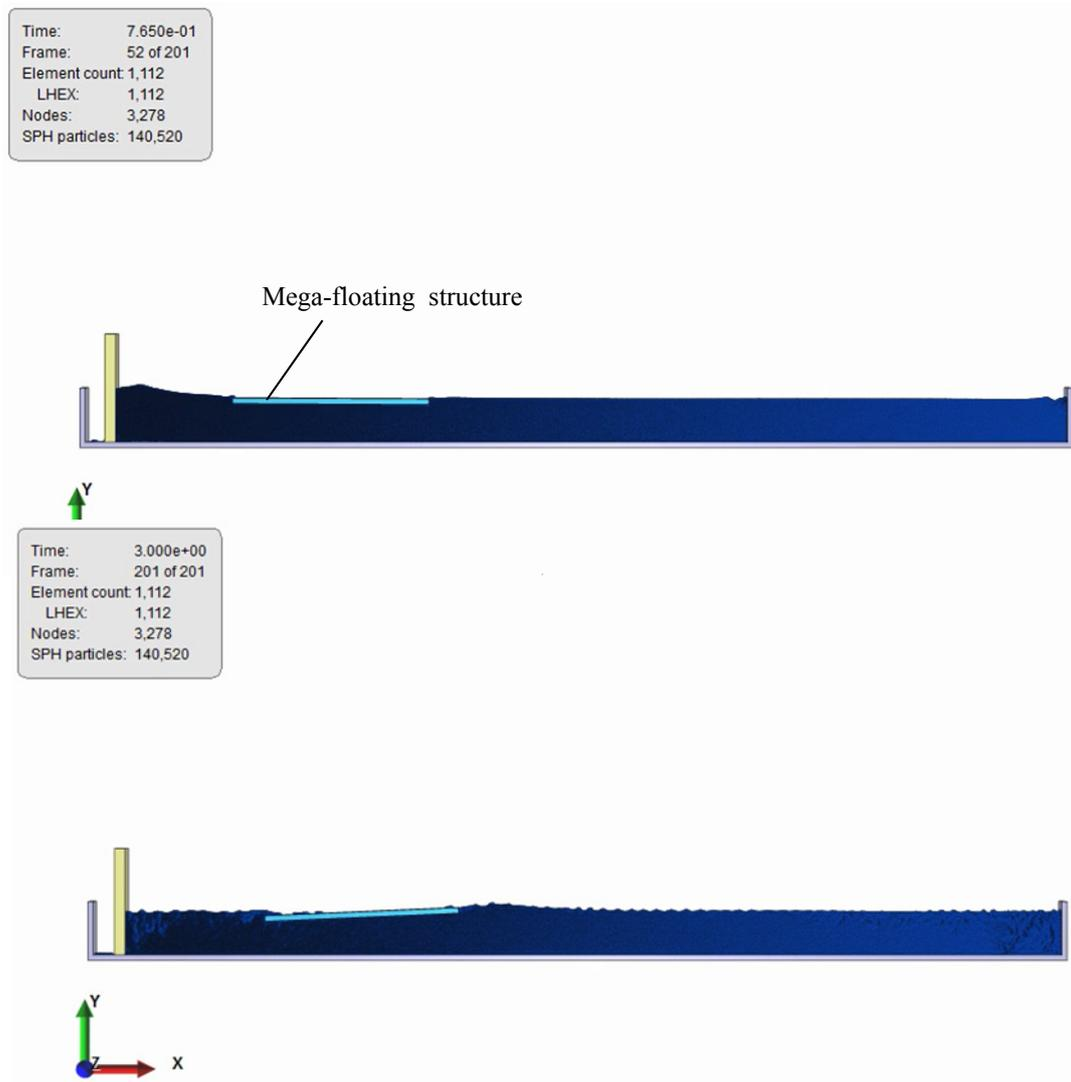
Figure 1 SPH computational results of the FSI between tsunami and mega-floating structure
