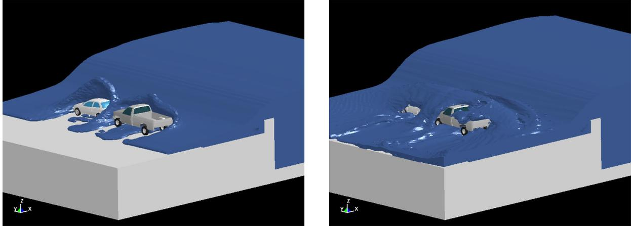
Fig. 2. Computational results of the tsunami behavior getting over the breakwater, and its attacking behavior on two vehicles.
