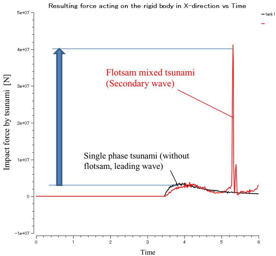
Fig. 9. Effect of flotsam mixing with tsunami on the impact force with a land structure.
