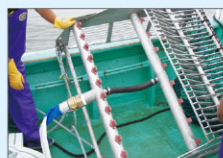
Water jet dredge
